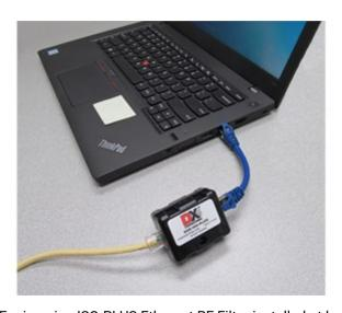
DX Engineering ISO-PLUS Ethernet RF Filter installed at laptop
