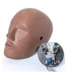
The A64C mounts on standard triaxial accelerometer mounting blocks and locations.
