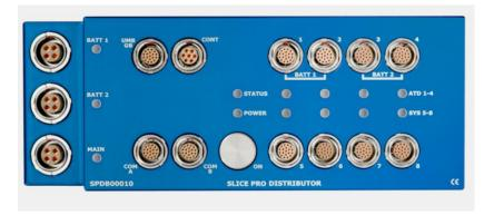
The LED indicators make it easy to manage individual system status and power status for high-channel count tests. The SLICE PRO DISTRIBUTOR output power of 588 W supports a mix of up to 820 channels of in-dummy and SLICE PRO DAS.
