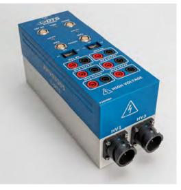
Compact and flexible, the FMVSS305 test unit can be used independently with manually operated switches or integrated with SLICE or TDAS data acquisition systems using standard DTS communication and power interfaces with DataPRO Software.
