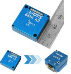
The miniature 6DX A2 measures high rates of acceleration and angular velocity and is designed for test articles with tight space constraints. The 6DX A2 mounts directly to the DTS SLICE6 data acquisition system via a built-in Nano-Strip connector which eliminates all sensor cabling.
