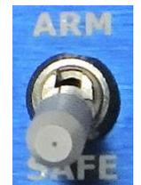
It is also possible to connect multiple ARM inputs in parallel and use a long cable (e.g., 70 m) to ARM enable the TOM. If you have questions about your specific application, contact DTS.
