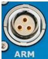
The TOM must be hardware enabled to arm and fire the squib channels. (The squib outputs are shorted when the unit is not hardware enabled.) To hardware enable your TOM, install the ARM Enable Plug provided or move the toggle switch to the ARM position (pull out on the switch to move—*do not force*).
