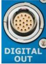
Each SLICE PRO TOM contains 8 independent and fully isolated digital output channels<sup>2</sup>. (See Appendix E for digital output drive strength.) Each channel may be configured individually via software for contact closure (normally open or normally closed) or 5 V TTL logic mode signals. In either mode, these channels are not powered and remain in a high-impedance state whenever the module is idle, not armed or the data collection time window has passed.
