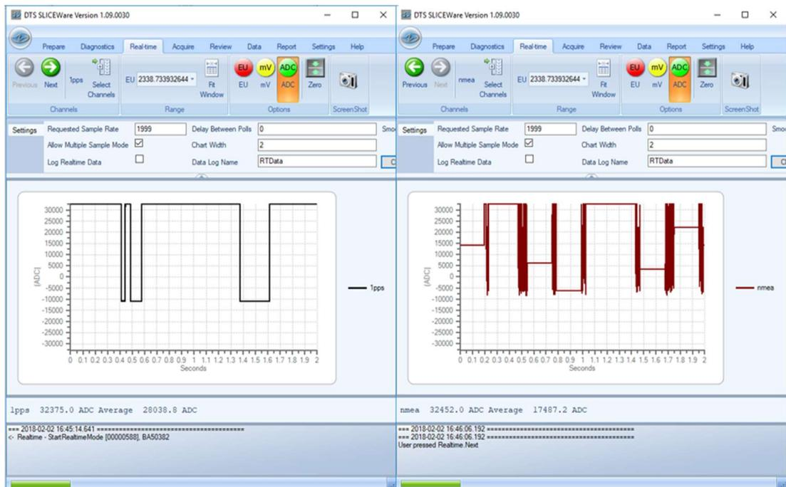
Figure 8: 1PPS and NMEA Signals in Real-time view
