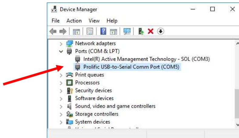
Figure 17: Windows Device Manager, USB-to-Serial Adapter COM5
