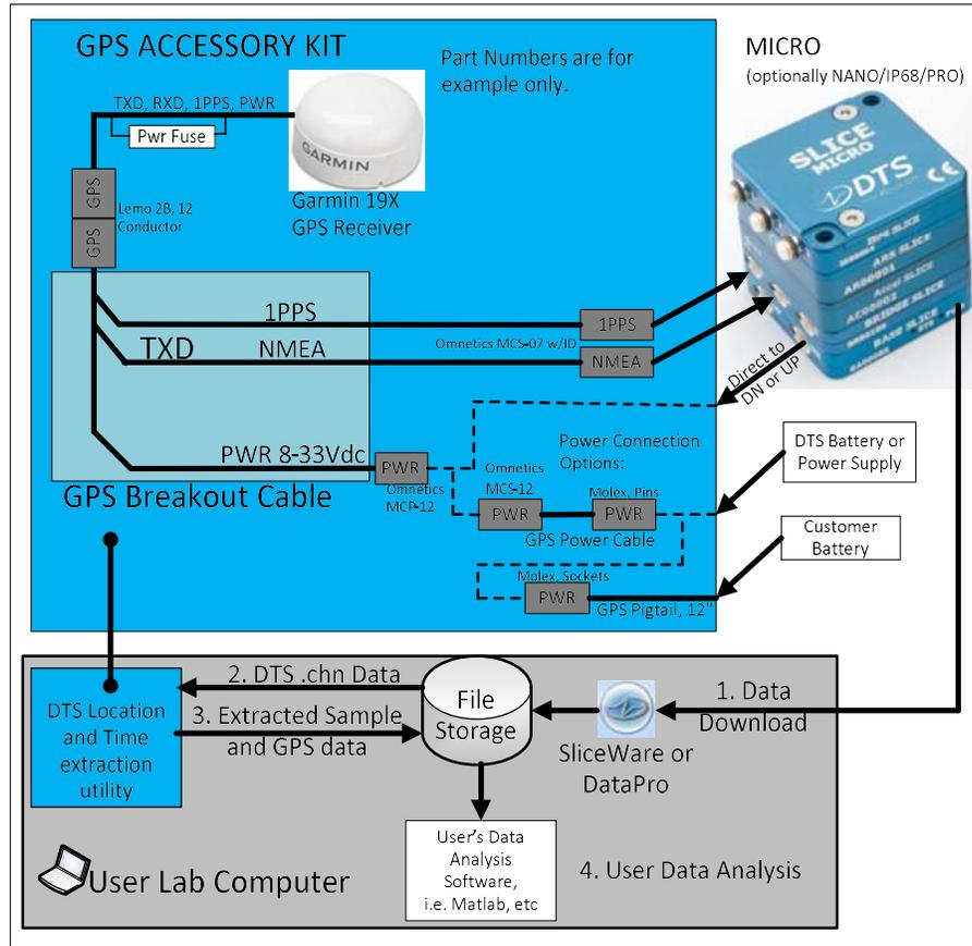
Figure 2: System Block Diagram, Hardware and Software
