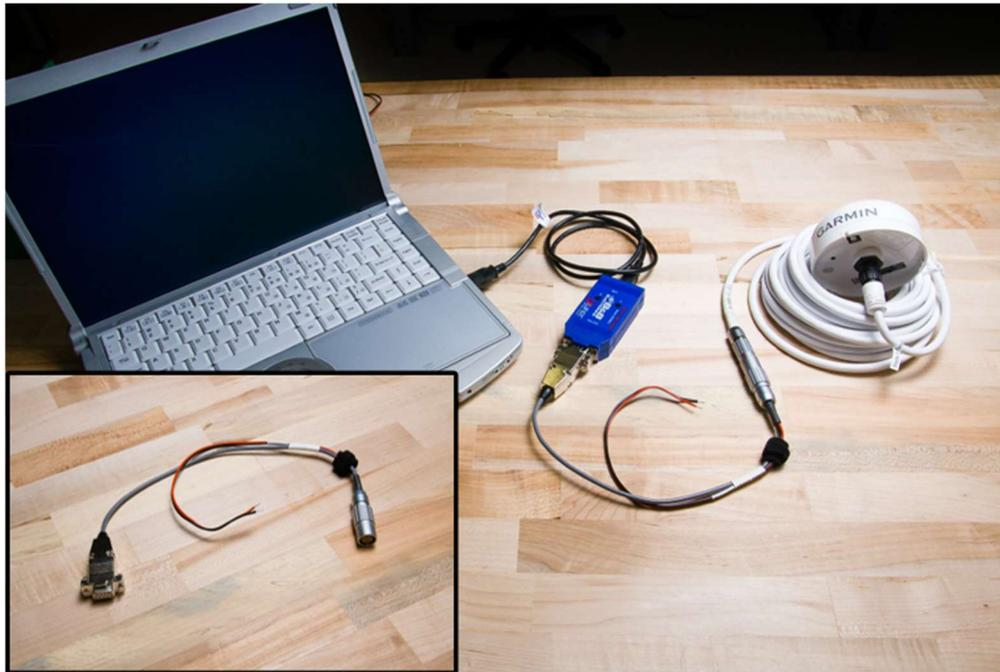
**Figure 18: GPS Receiver Configuration Connection**
