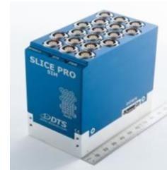
The SLICE PRO SIM is available with either 9 or 18 (as shown) fully-programmable sensor input channels that provide power and signal conditioning to support a variety of external sensors.
