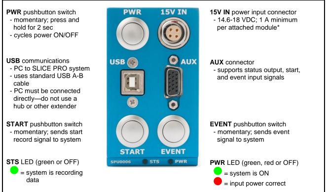
A minimum of 500 mA per module is needed to charge the internal back-up batteries of attached modules. (Controllers are considered modules for the purposes of power calculations.) Be sure to consider any power drop due to cable length.
