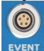
Some TDAS PRO racks are configured so they may be powered on and off remotely via the EVENT connector. This has the same effect as using the ON power switch. A normally open momentary switch should be used for this purpose. The system will power up and remain on as long as the signal is applied and will power down when the signal is absent for at least 3 seconds.
