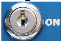
A key switch is used for on/off control. Total time from ON initiation to system ready is ~10 seconds. Multiple units in a chain may be started in any order, however be sure to wait at least 10 seconds between each rack to avoid communication conflicts. When the power LED on the modules are blinking green, you may start the software.
