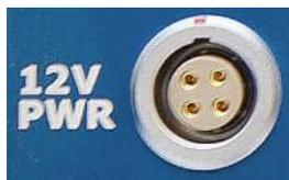
External power is provided via the 4-pin 12V PWR connector and is used to 1) charge all TDAS PRO system batteries (rack and modules) when system power is off, or 2) simultaneously charge and run a TDAS PRO system when system power is on. If input power fails, the system will transition to internal battery reserves.
