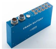
Compact and ruggedized, the Crash Battery provides pass-through power and battery backup for TDAS PLUS Mini Distributor, TDAS PRO, TDAS G5, and SLICE data acquisition systems.
