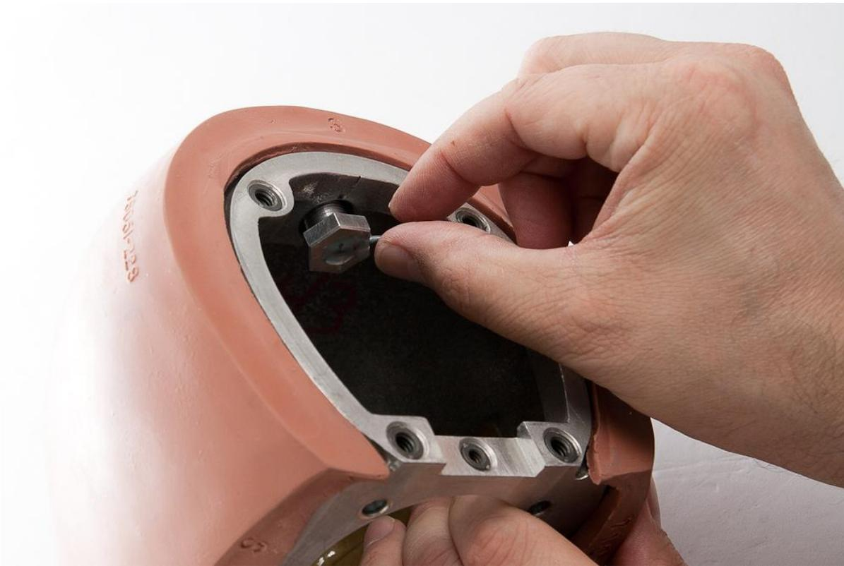
4. Insert neck load cell structural replacement into skull. Note the position of the flat edge relative to the FMH skull.
