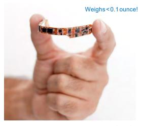
The DDR is a standalone 6-degrees-of-freedom (6DOF) data logger that measures linear and angular acceleration. The ultra-light logger is designed to monitor short duration events in small devices under test.
