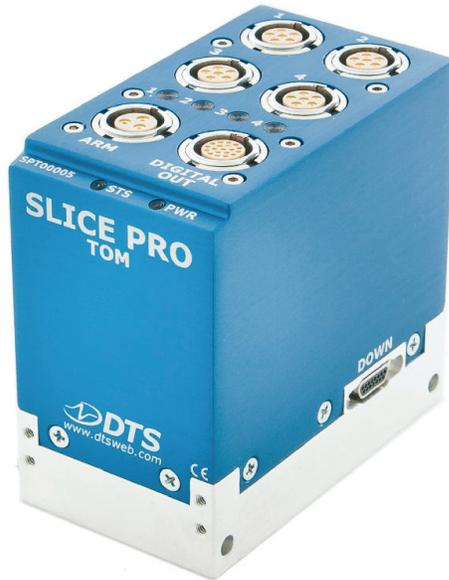
Each SLICE PRO TOM fires up to 4 pyrotechnic devices with squib firing delays from 0 to 99 seconds with 0.1msec resolution. Need more TOM channels? Simply add more modules.
