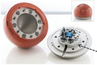
The SLICE Pedestrian Headform Impactor features an integrated 3-channel SLICE NANO data acquisition system and a triaxial accelerometer (shown with a DTS ACC3). Embedding the data recorder eliminates trailing cables that may get tangled or cause issues with noise or data loss. The turn-key solution is engineered to maintain proper mass, center of gravity (CG) and moments.
