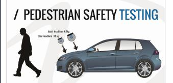
The SLICE Pedestrian Headform Impactor integrates the ultra-small SLICE NANO data acquisition system into a cable-free solution for pedestrian safety testing. Offering the ultimate in flexibility and reliability, the headform is armed via a PC, disconnected, then powered and launched any time without trailing cables. The system can be triggered with a level trigger or contact closure and writes data to flash memory.
