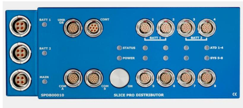
The LED indicators make it easy to manage individual system status and power status for high-channel count tests. The SLICE PRO DISTRIBUTOR output power of 588 W supports a mix of up to 820 channels of in-dummy and SLICE PRO DAS.
