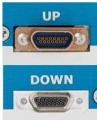
The UP interface connector allows the user to interface to a SLICE PRO Ethernet Controller, USB Controller or another SLICE PRO module. (The UP connector may appear loose, however do not tighten.) The DOWN interface connector allows the user to interface to another SLICE PRO module (chainable with up to 3 other modules). Please see Appendix B for pin assignments.
