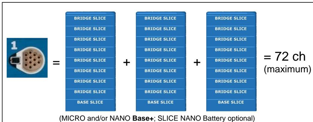
Maximum current for all 4 SLICE System connectors combined is 10 A with a maximum of 4 A per connector. Carefully calculate your expected maximum power consumption to ensure compliance with power limits. (Please see page 9 for information on power requirements.)
