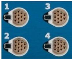
These 4 connectors are identical and support power, start, event, status and USB communication signals for the DAS. One SLICE connector supports up to 3 SLICE stacks, with a maximum of 8 SLICE Bridges per stack, in any combination of SLICE MICRO or NANO. SLICE MICRO Accel and ARS units can be used in place of a Bridge and the SLICE NANO Battery can be used with any SLICE NANO stack.
