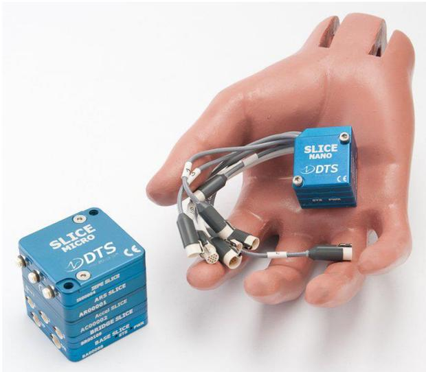
SLICE MICRO and SLICE NANO are standalone, user-configurable data acquisition systems designed for extreme test environments. SLICE MICRO and NANO support a variety of external sensors to measure acceleration, strain, voltage, temperature and more.
