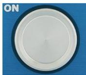
A low-profile piezo switch is used for on/off control. There is no detectable movement in the switch; you must press and hold firmly for 2 seconds to start or stop the system. Total time from ON initiation to system ready is typically between 1-2 minutes. Multiple units in a chain may be started in any order. Be sure to follow proper procedures to avoid an unstable condition.
