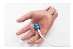
Each sensor cable is 7 meters (23 feet) long and terminates to a single triaxial connector. Pigtail or adapter cables are available to support a variety of termination options.
